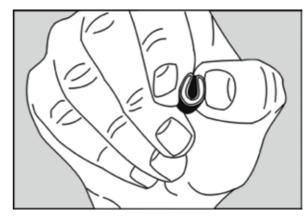
Folding the tube seal for insertion into the membrane.
