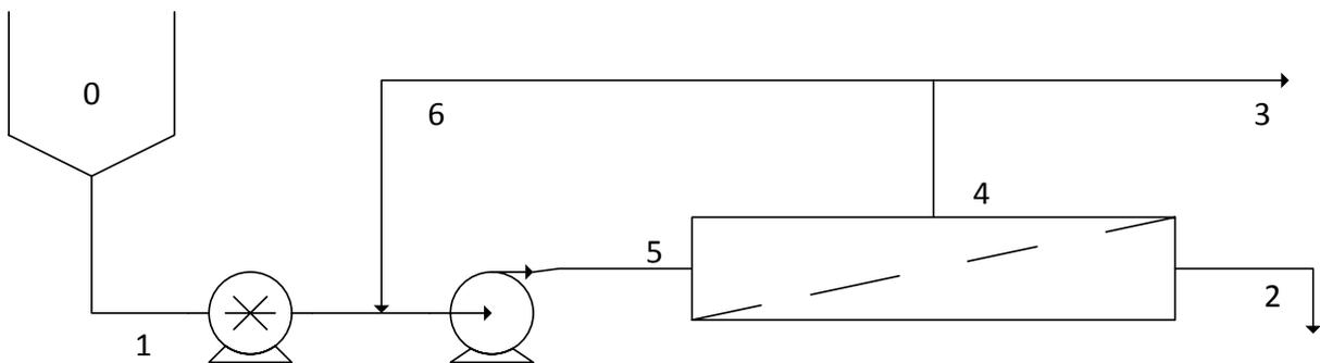
Once through system design with feed and recycle pump.
